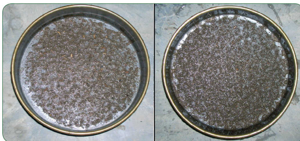
FIGURE 2.26. Pictures of different soil aggregate test results: A Lima silt loam soil from a long-term tillage experiment. (Left) Moldboard plow treatment with 34% water stable aggregates. (Right) Zone-till management with 56% water stable aggregates (0.25 mm sieve).
