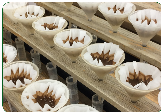
FIGURE 2.41. Potentially Mineralizable Nitrogen (PMN) processed in the lab. The difference between pre-incubation and post-incubation ammonium measurements is used as an indicator of N mineralization.
